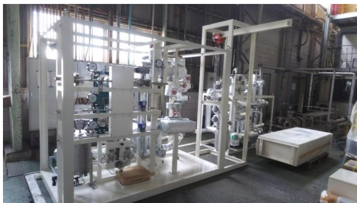
Bench Scale Test 1.25Nm 3 -CH 4 /h (IHI Yokohama Engineering Center)
