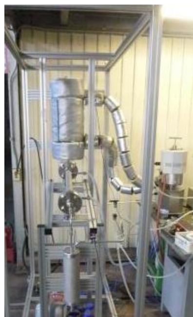
Lab Scale Test ~0.05Nm 3 -CH 4 /h (IHI Yokohama Engineering Center)
